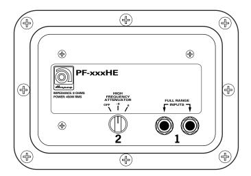
1. 1/4" TS Full Range Input / Output Jacks: The jackplate features two 1/4" jacks wired in parallel, allowing easy daisy-chaining from one speaker to another. Each of the jacks may be used as an input or a through connection.
